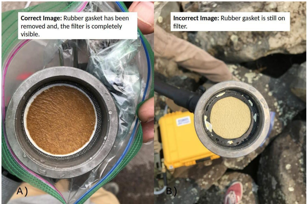
FIGURE A.7 A = this is the correct image; the rubber gasket has been removed, and the filter is completely visible. B = this is the incorrect image; the rubber gasket is still on the filter.
