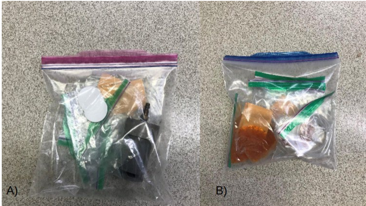
FIGURE A.4. Infographic showing the recommended organization of consumables for eDNA field sample collection with the OSMOS and the DIY peristaltic pump. Each station's consumables are placed into a single large plastic bag, clearly labeled with the station ID for easy identification and organization: A = OSMOS sampling bag containing a loaded filter cartridge, forceps, three filters for the biological replicates, and three coin envelopes in desiccated silica for the biological replicates; B = DIY peristaltic pump sampling bag containing sterile forceps, tubing, four filters, three coin envelopes for desiccated silica for the biological replicates, and one coin envelope in desiccated silica for the negative control (GEN-FISH 2022b, 2022d). Such organization is critical for efficient and accurate eDNA sample collection.
